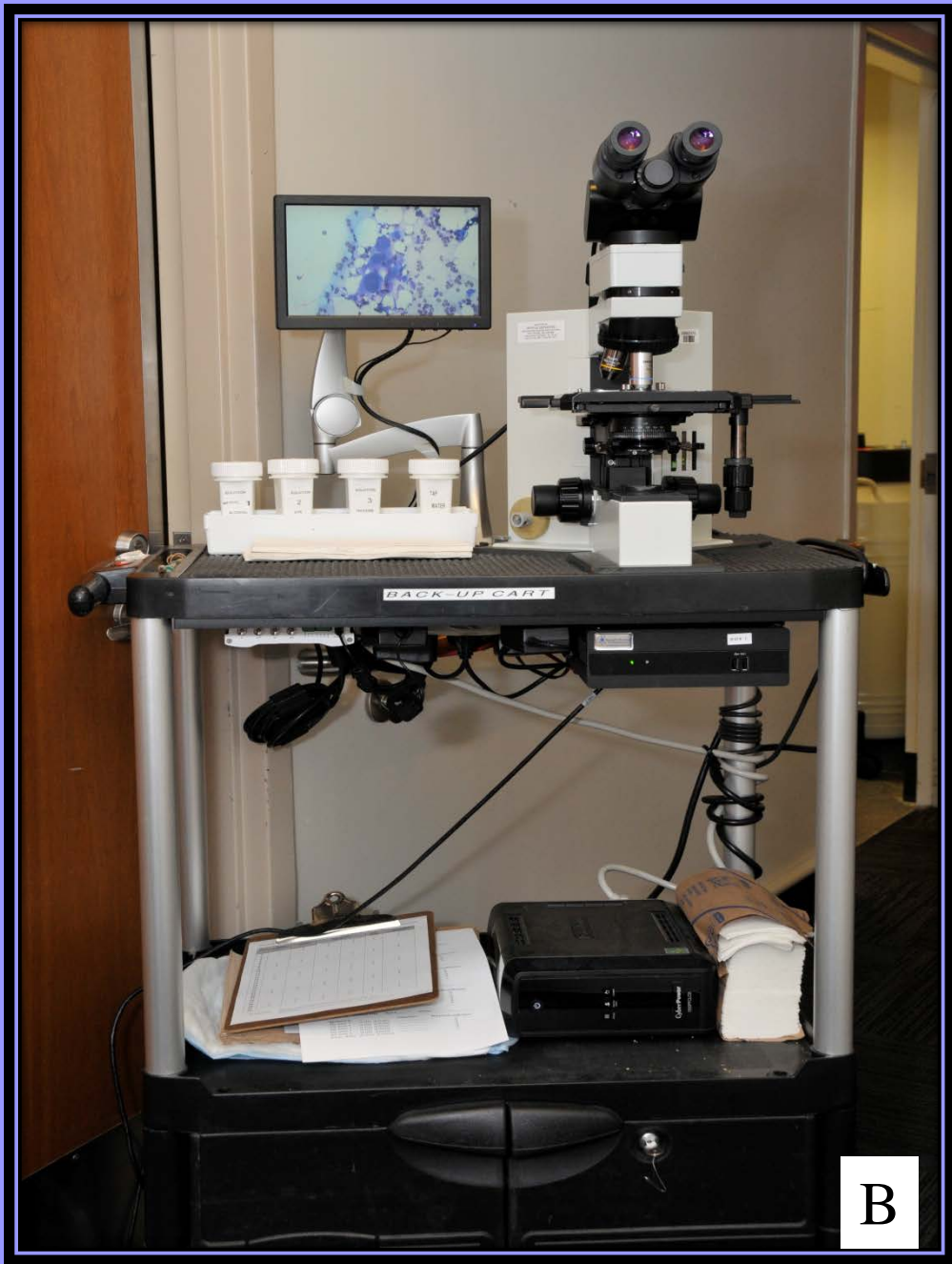
Figure 2 RMT system. A) fixed location B) Mobile cart
